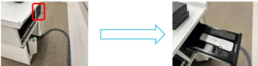
2. Connect the USB cable prepared in step 1 to the 【USB (Audio)】 port on the operation desk.
