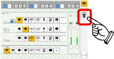
2. On the touch panel, go to the main control screen > [Video Source Selection] > select USB Capture Sending to **【Camera】** , and confirm that the camera image appears on the preview monitor on the desk.
