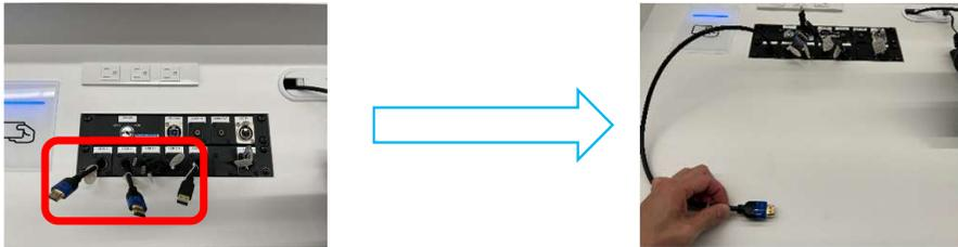
3. On the touch panel, go to the main control screen > **【Video Source Selection】** > select projector **【HDMI1 (or HDMI2)】** , and the document camera's image will be displayed on the projector.
