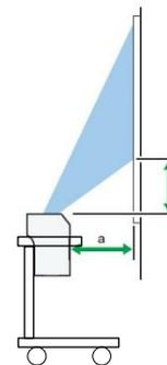
!! The projector screen size will change, according to the distance between the screen and the projector.
