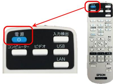
⇒ **Press ON/OFF Power button** on the remote control and system will be turned on.
