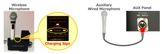
Make sure to return to the microphone charger after using the microphone.
