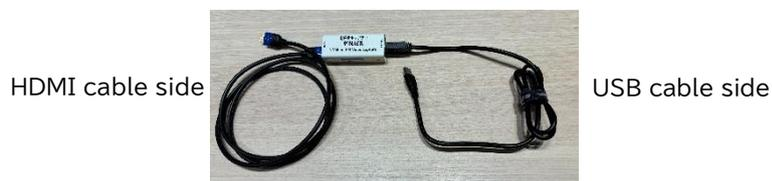
2. Connect the HDMI cable side connected in step 1 to **[PJ OUT]** on the **console**, and connect the USB cable side to the PC
