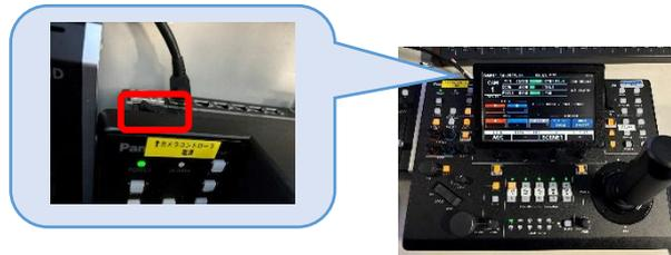
4. Turn off the power on the cart at the bottom right of the console.
