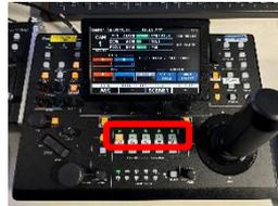
2. While checking the console monitor(existing), move the stick to pan/tilt.
