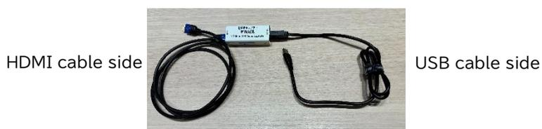
2. Connect the HDMI cable side connected in step 1 to **[CAM OUT] on the console**, and connect the USB cable side to the PC
