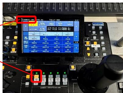
4. **While holding down the [F1],** touch the number to register as a preset on the controller's main monitor (Here, touch PRE6)
