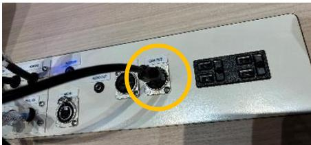
Connect the HDMI terminal to [CAM OUT]
