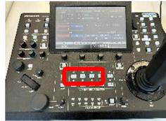
2. While checking the monitor screen for the live switcher, move the stick to pan/tilt
