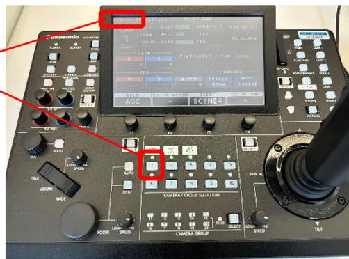
4. While holding down the [F1], touch the number to register as a preset on the controller's main monitor (In this case, touch PRE6)
